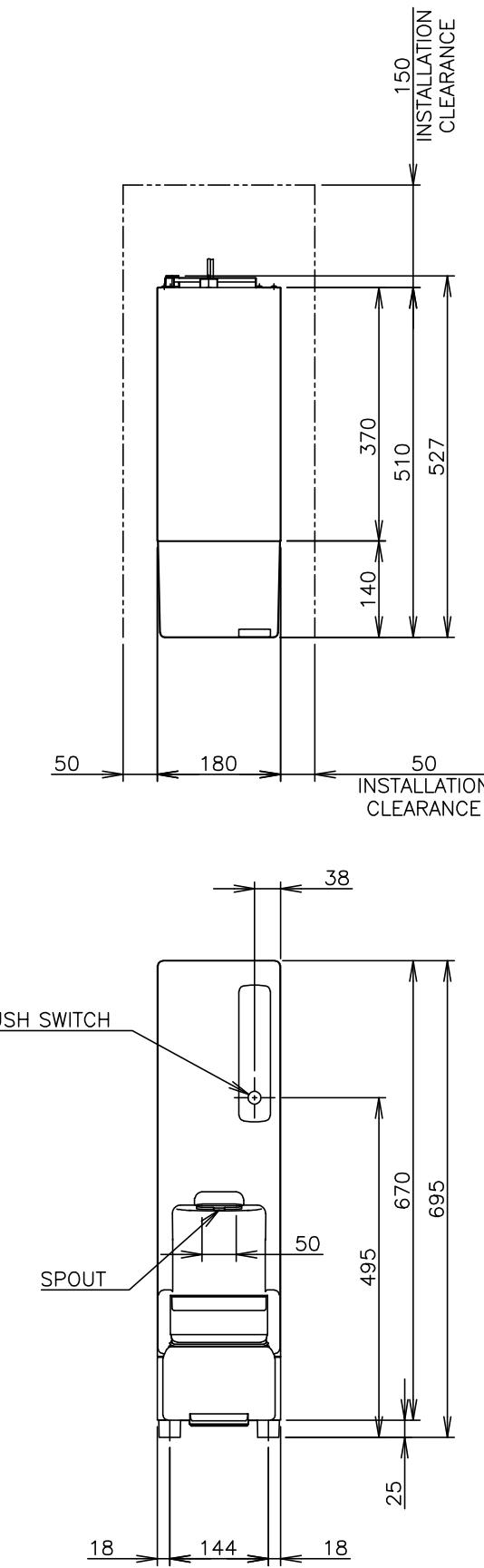
1. Install the product properly in accordance with the instructions on location, electrical connections stated in the instruction manual provided. Allow 10mm extra space at the installation site to meet any installation requirements (additional spacing is also required for proper air flow).
