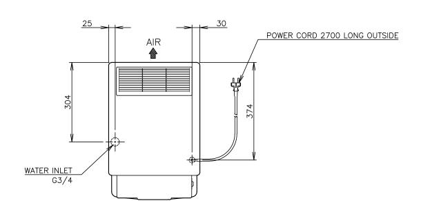
Ambient Temp.: 5-40°C, Water Supply Temp.: 5-35°C
